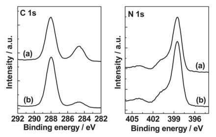
Figure 7. C 1s and N 1s XPS spectra of: a) bulk g-C<sub>3</sub>N<sub>4</sub>, and b) g-C<sub>3</sub>N<sub>4</sub> nanosheets. The peak of C 1s at 284.6 eV arises from the adventitious carbon in the samples.
