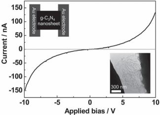
**Figure 9.** Typical I-V curve of a single g-C<sub>3</sub>N<sub>4</sub> nanosheet. The insets are the schematic (the upper left panel) and the TEM image (the bottom right panel) of the single nanosheet between two Au electrodes.
