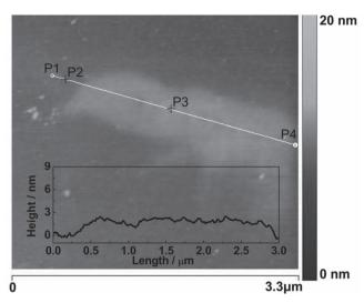
Figure 3. Tapping-mode AFM image of a single g- $C_3N_4$  nanosheet deposited on the silicon wafer substrate. The inset is the height curve determined along the line between P1 and P4.
