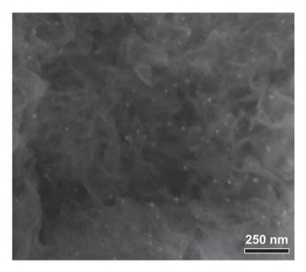
Figure 12. SEM image of g- $C_3N_4$  nanosheets collected after photocatalytic hydrogen evolution reaction.
