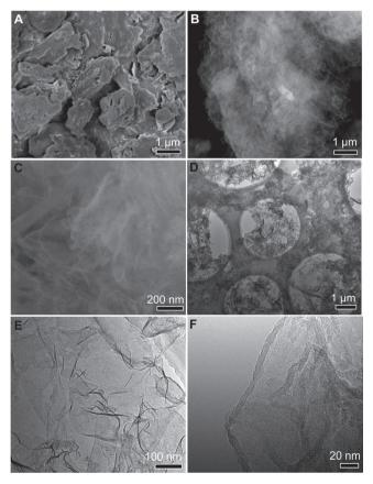
**Figure 2.** A) SEM image of bulk g- $C_3N_4$ . Low- (B) and high-magnification (C) SEM images of representative agglomerates of g- $C_3N_4$  nanosheets. Low- (D) and high-magnification (E) TEM images of g- $C_3N_4$  nanosheets. F) TEM image of the sheet edge area of g- $C_3N_4$  nanosheets.
