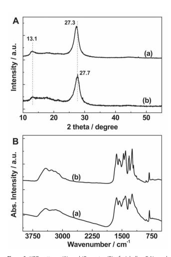
Figure 6. XRD patterns (A), and IR spectra (B) of: a) bulk g-C $_3N_4$ , and b) g-C $_3N_4$  nanosheets.
