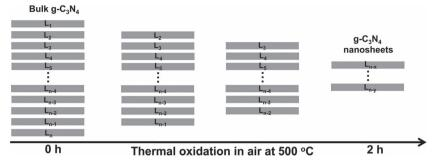
**Figure 5.** Schematic of the formation process of the g- $C_3N_4$  nanosheets by thermal oxidation etching of bulk g- $C_3N_4$  at 500 °C in air.
