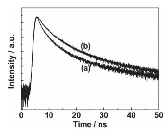
**Figure 10.** Time-resolved fluorescence decay spectra of a) bulk  $g-C_3N_4$ , and b)  $g-C_3N_4$  nanosheets monitored at 468 and 448 nm, respectively, by time-correlated single-photon counting. The samples were excited by the incident light of 330 nm from a picosecond pulsed light-emitting diode.
