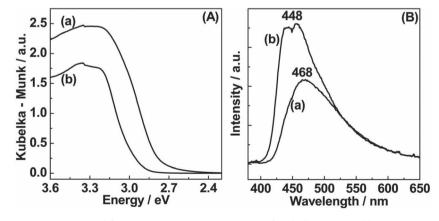
Figure 8. UV-visible absorption spectra (A) and fluorescence emission spectra (B) of: a) bulk g-C<sub>3</sub>N<sub>4</sub> and b) g-C<sub>3</sub>N<sub>4</sub> nanosheets. The wavelength of excitation light for fluorescence emission spectra is 350 nm.
