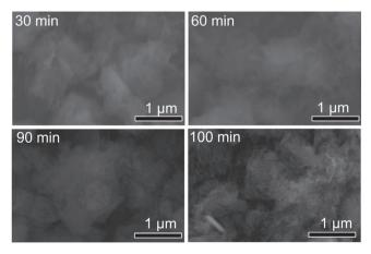
Figure 4. Morphology evolution of bulk g- $C_3N_4$  with the increased thermal oxidation etching time at 500  $^{\circ}C$  in air.
