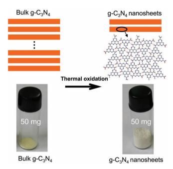
**Figure 1.** Schematic of the structures of the bulk g- $C_3N_4$  and the g- $C_3N_4$  nanosheets. Carbon, nitrogen, and hydrogen atoms are respectively indicated by grey, blue and red spheres in the atomic model. A volume comparison of 50 mg powder of bulk g- $C_3N_4$  and g- $C_3N_4$  nanosheets is given.
